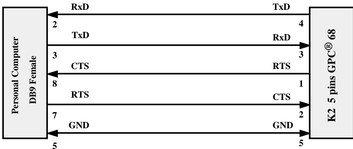
SERIAL CONNECTION BETWEEN P.C. AND BOARD THROUGH 6 PINS PLUG CONNECTOR
